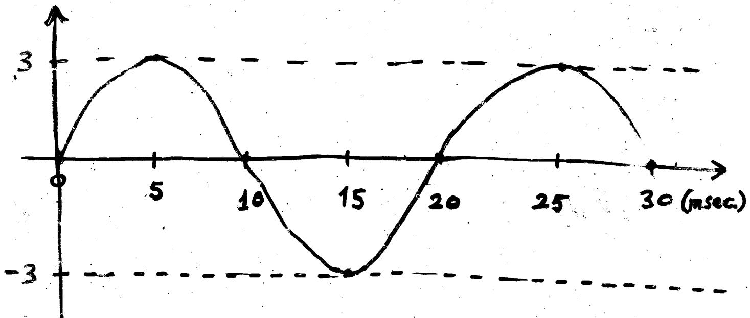
b) The signal  $x_a(t)$  is sampled with a sampling rate  $F_s = 300 \text{ samples/sec.}$  Determine the frequency of the discrete-time signal  $x[n] = x_a(nT_s)$ ,  $T_s = \frac{1}{F_s}$  and show that  $x[n]$  is periodic.
