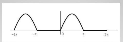
$\label{eq:Vout} V_{out}(t) = \begin{cases} sin(\omega t) & 0 < \omega t < \pi \\ 0 & \pi < \omega t < 2\pi \end{cases}$
